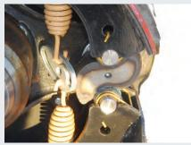
Axle Notes - On our QM-14, QM-1400, QM-16, OM-1600 and OM-1800 models 10 stud 120mm 420x180 S-Cam commercial axles are standard. This is the same size of axle used by HGVs.
